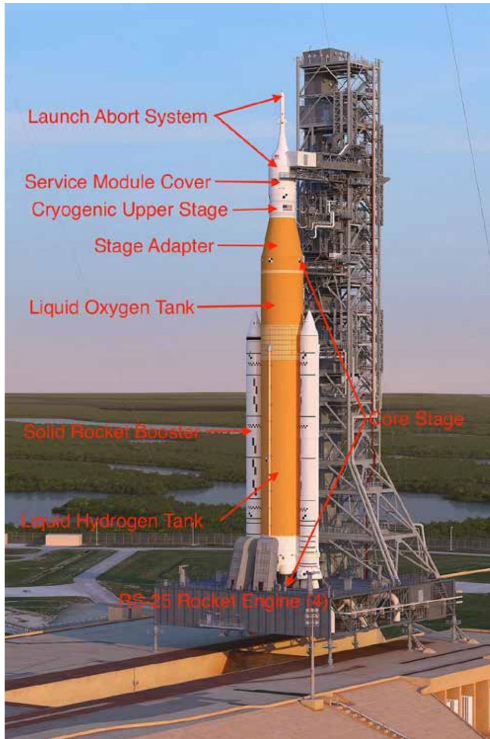
Space Launch System, Block 1 (early version) with major components identified—note that the RS-25 engines are mounted below the core stage and are not clearly visible (this represents the configuration that will perform a lunar fly-by with astronauts on board, but will not land)
