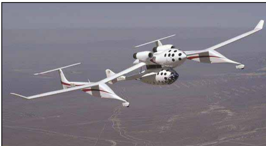
The aerospace “mother ship,” known as “White Knight” is shown here carrying SpaceShipOne on a test flight. Image courtesy of Mojave Aerospace Ventures, LLC
