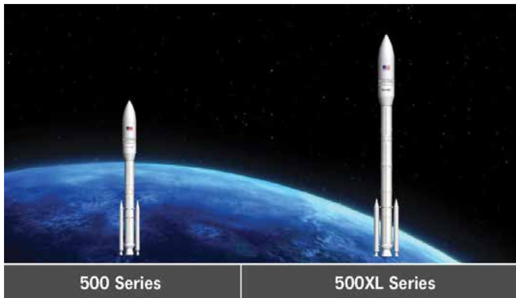
Omega Rocket: Size comparison of the two versions of the rocket; the more powerful version will use a central core based on a full-size Space Shuttle Solid Rocket Booster
