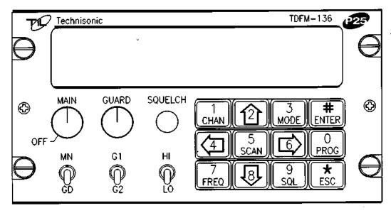
MAIN – Main channel volume and power on/off switch GUARD – Guard channel volume SQUELCH – Squelch defeat
